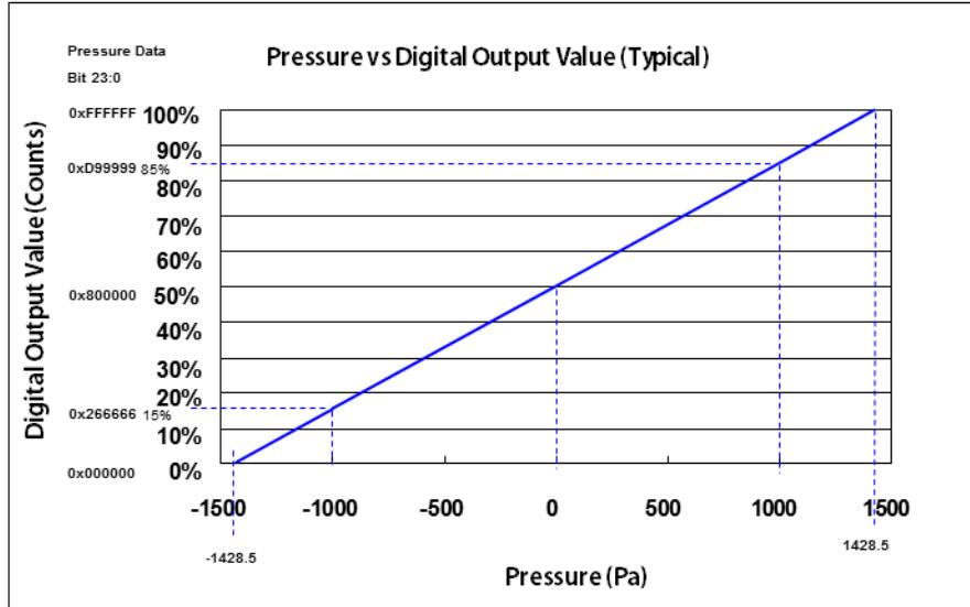
$$P_{out} (\text{Pa}) = \frac{(\text{ADC Value}_{(\text{Bit } 23:0)} - 0x800000_{\text{HEX}}) * (0x07d0_{\text{HEX}})}{(0xb33333_{\text{HEX}})}$$
